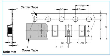
Carrier tape transparent cover tape should be heat-sealed to carry the products, and the reel should be used to reel the carrier tape.
