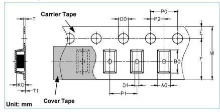
Carrier tape transparent cover tape should be heat-sealed to carry the products, and the reel should be used to reel the carrier tape.
