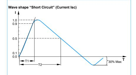
IEC 61000-4-2 Compliant ESD Current Pulse Waveform
