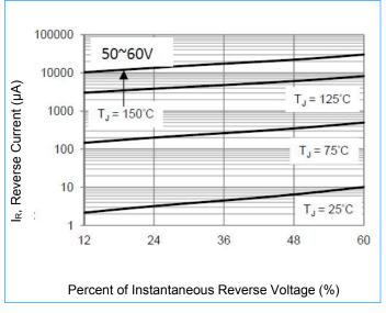
Fig8. Typical Reverse Characteristics
